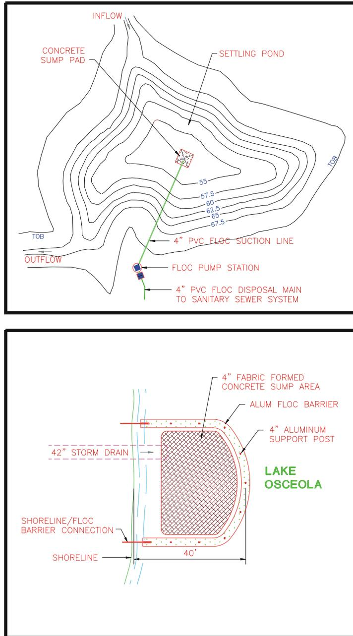
Figure 4. Typical schematics of floc collection and disposal systems
