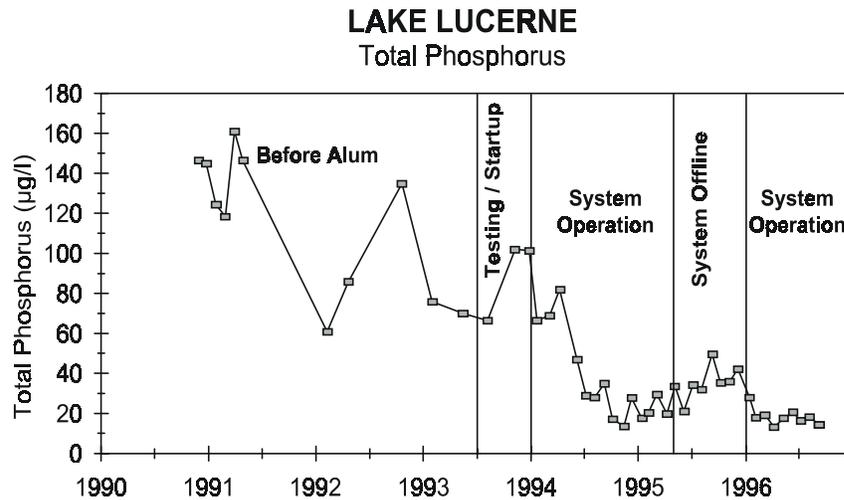
Figure 1. Trends in total phosphorus concentrations in Lake Lucerne, before and after alum treatment of stormwater runoff
