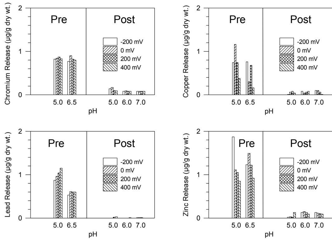
Figure 3. Comparison of sediment-metal phase in pre- and post-treatment sediments in Lake Ella
